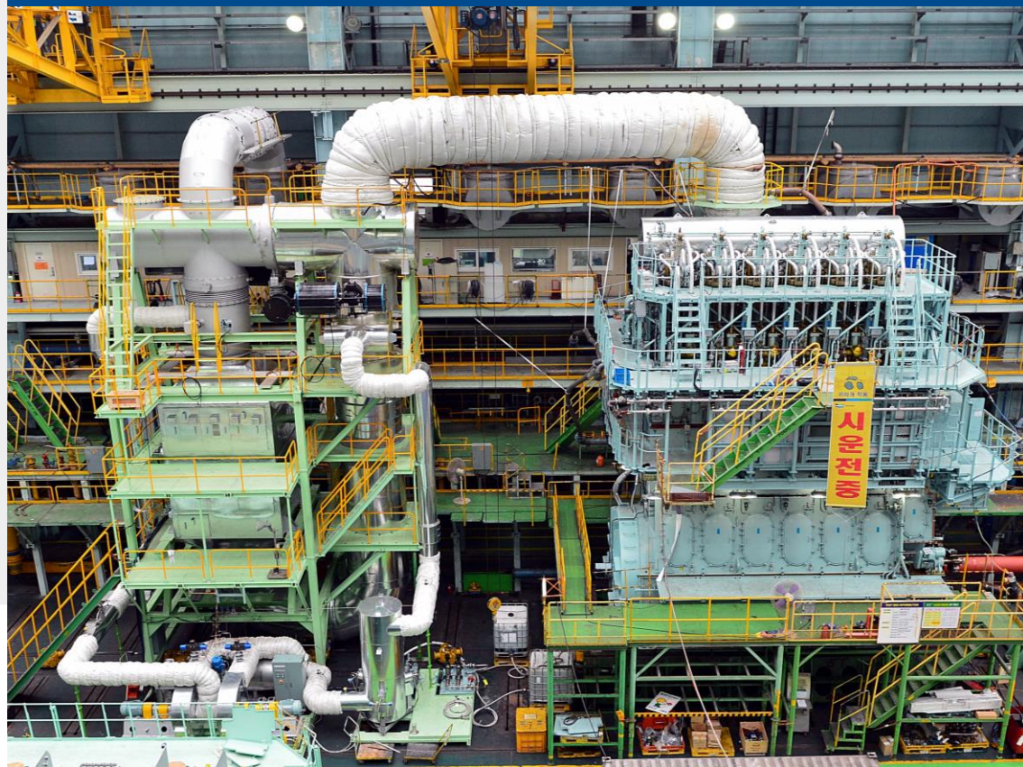
Slow revolving 2-stroke engine with SCR system under construction (picture Hyundai Heavy Industries)
